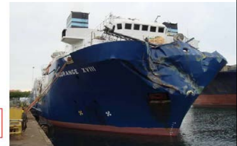
Photo 4: Damage to Big Orange XVIII (source: ConocoPhillips)
