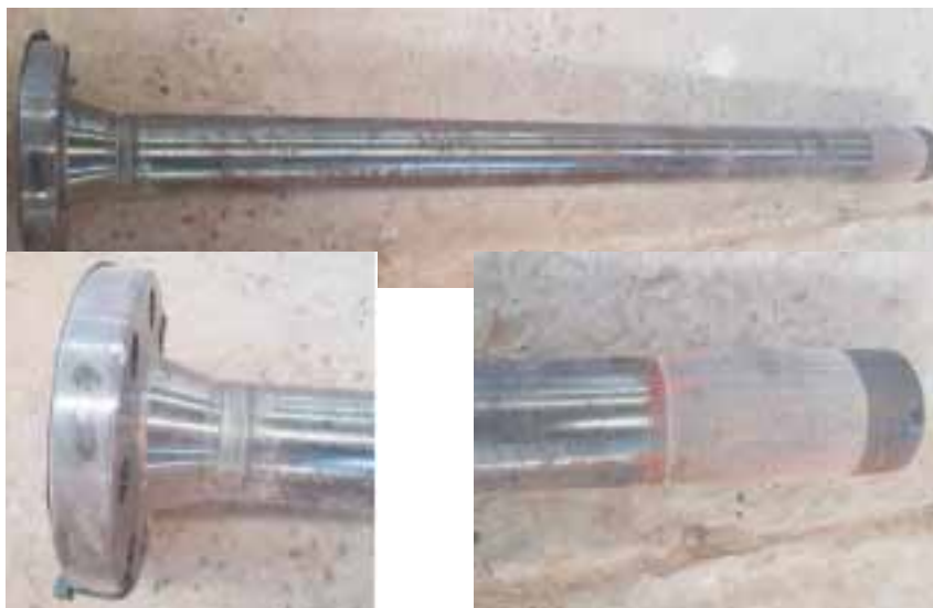
Figura 11. Crossover brida welded neck a Box Stealth Lock.
