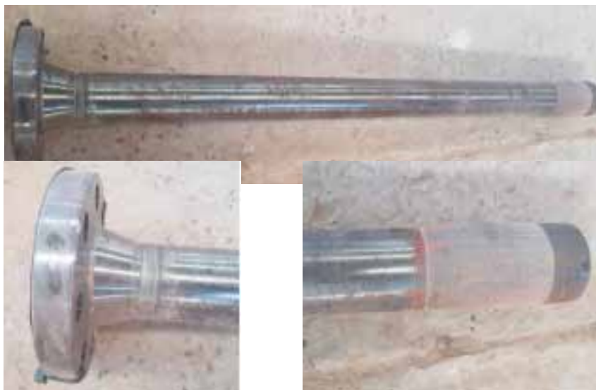
Figura 11. Crossover brida welded neck a Box Stealth Lock.
