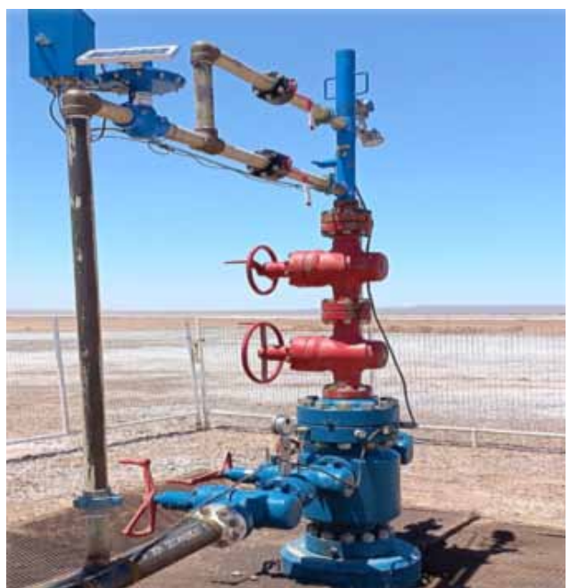
Figura 14. Plunger lift en shale oil de PAE.
